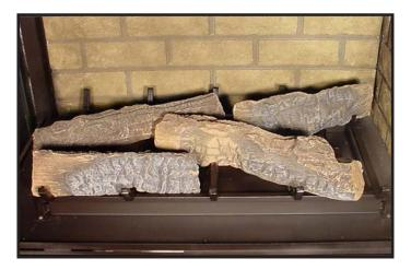
**LOG #4 (SRV2068-703):** Place log #4 in the left front corner of the log grate using bottom grooves for placement. Align log #4 by using the grate corner and front cross bar as stops.
